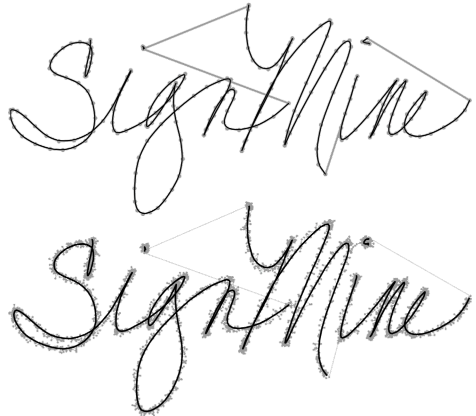
Tangential (upper panel) and smoothing (lower panel) interpolations with a quadratic kernel
